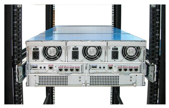
14. Use six (6) M5 screws to lock the enclosure into the rack post, one screw in each corner. Note that the screw driver will need to pass through the corner hole of front panel for the two upper corner holes on both sides.
