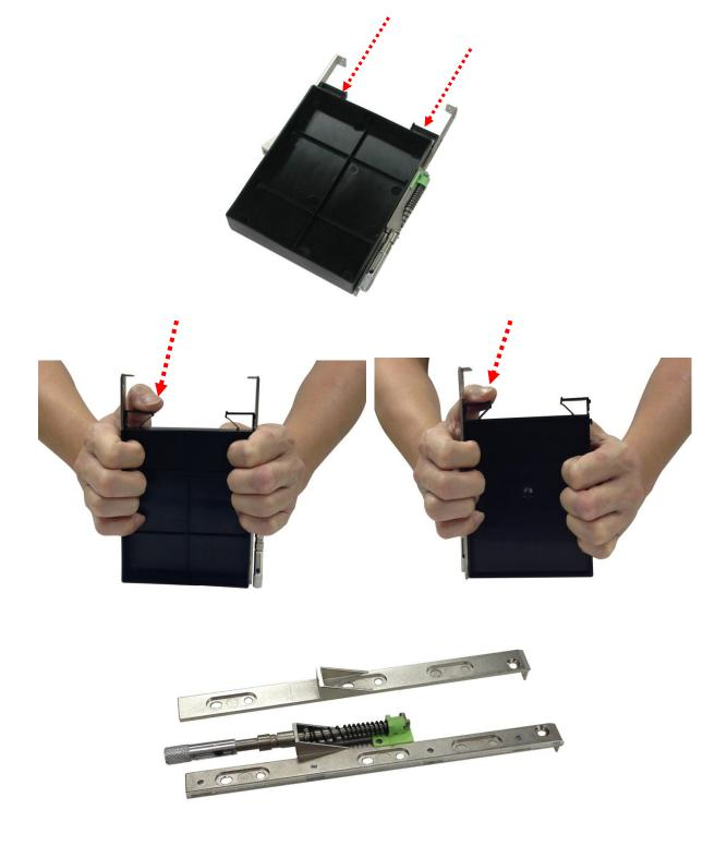
2. Place the brackets on both sides of the disk drive and secure them with screws.
