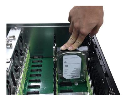
4. Tighten the thumbscrews on the sides of the disk drive.
