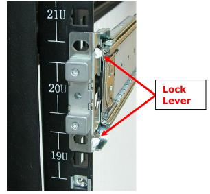
View from Front Side of Front Left Rack Post Lock Lever is Locked
