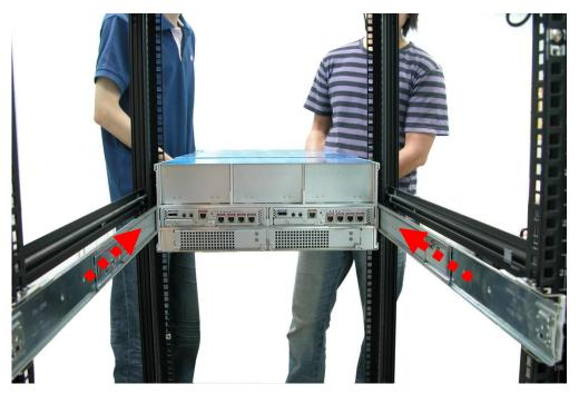
4. Push the white lock to release the subsystem from the rail.
