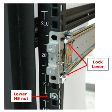
View from Front Side of Front Left Rack Post Lock Lever is Not Locked
