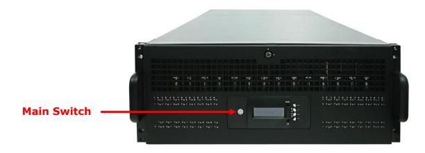
4. Allow the machine a few moments to initialize before using it. The main switch button will continue flashing blue until the system is finished checking each disk slot.
