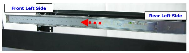
Middle Rail Member of Rail Assembly on Left Side of Rack
