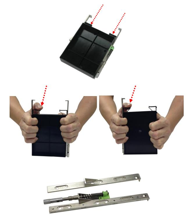
2. Place the brackets on both sides of the disk drive and secure them with screws.
