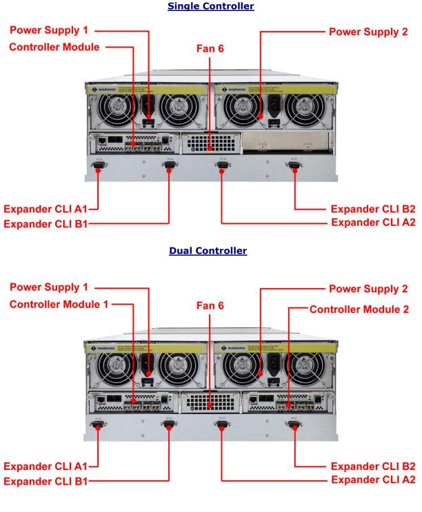
NOTE: Each Power Supply Module has 1 Power Supply and 5 Fans. For purpose of hardware monitoring, the RAID enclosure is logically divided into two enclosures.
