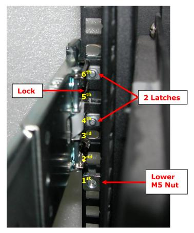
View from Rear Side of Front Left Rack Post 2 Latches are inserted in the 4<sup>th</sup> and 6<sup>th</sup> holes from bottom (M5 nut) 7. Install the other end of rail assembly to the left rear side. Align and insert the 2 latches on the 2 holes on the rear rack post, and then push the rail a little towards the rear side and lock the lock lever on the rack post.
