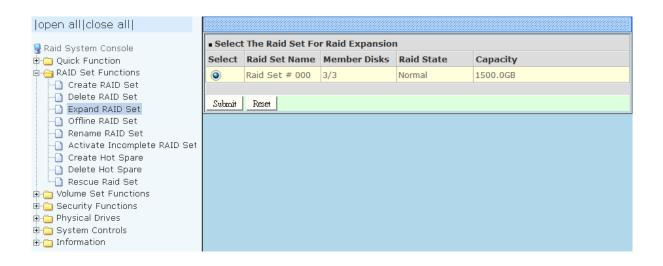
To expand a Raid Set, click on the **Expand RAID Set** link. Select the Raid Set which you want to expand.
