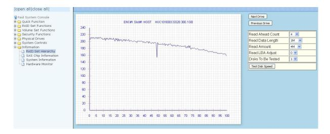
If there's a certain location in the hard drive that is getting poor performance, hard drive read benchmarks can help confirm this. Above is a screenshot of a palimpsest benchmark on a hard drive. The length time of firmware takes to complete the drive test depends on its size.
