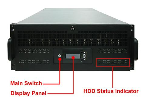
IMPORTANT: When powering off the Disk Array, turn off first the Main Switch and allow at least 4 minutes for the subsystem to shutdown properly. Then turn off the switches of the 2 Power Supply Fan Modules.
