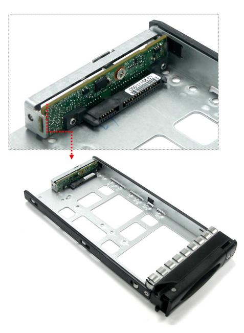
8. Place the Fixed Bracket with the dongle board in the disk tray as shown.
