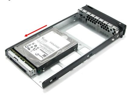
7. Turn the disk tray upside down. Align the four screw holes of the 2.5" SATA disk drive in the four *Hole y* of the disk tray. To secure the disk drive into the disk tray, tighten four screws on these holes of the disk tray. Note in the picture below where the screws should be placed in the disk tray holes.
