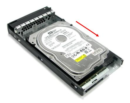
7. Turn the disk tray upside down. Align the four screw holes of the SATA disk drive in the four *Hole B* of the disk tray. To secure the disk drive into the disk tray, tighten four screws on these holes of the disk tray. Note in the picture below where the screws should be placed in the disk tray holes.
