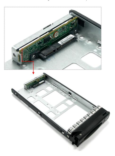
5. Turn the tray upside down. Align the holes of the Fixed Bracket in the two *Hole d* of the disk tray. Tighten two screws to secure the Fixed Bracket into the disk tray.
