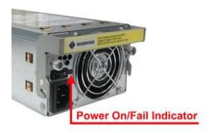
When the power cord connected from main power source is inserted to the AC Power Inlet, the power status LED becomes RED. When the switch of the PSFM is turned on, the LED will turn GREEN. When the Power On/Fail LED is GREEN, the PSFM is functioning normally.
