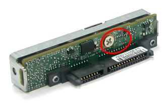
4. Place the Fixed Bracket with the dongle board in the disk tray as shown.
