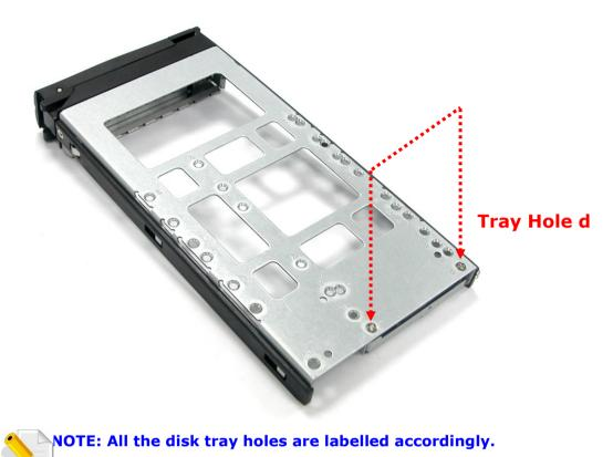
6. Place the 2.5" SATA disk drive into the disk tray. Slide the disk drive towards the dongle board.
