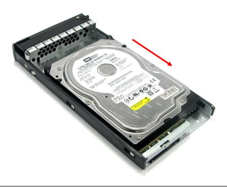
7. Turn the disk tray upside down. Align the four screw holes of the SATA disk drive in the four *Hole B* of the disk tray. To secure the disk drive into the disk tray, tighten four screws on these holes of the disk tray. Note in the picture below where the screws should be placed in the disk tray holes.
