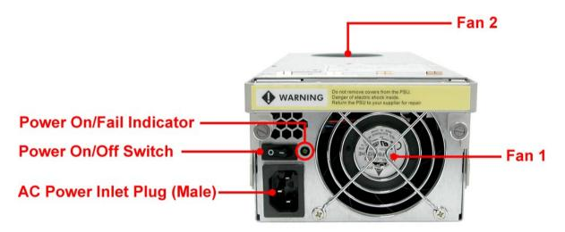
The panel of the Power Supply/Fan Module contains: the Power On/Off Switch, the AC Inlet Plug, and a Power On/Fail Indicator showing the Power Status LED, indicating ready or fail.
