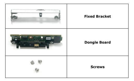
3. Attach the dongle board in the Fixed Bracket with a screw.
