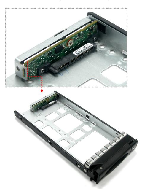
4. Place the Fixed Bracket with the dongle board in the disk tray as shown.
