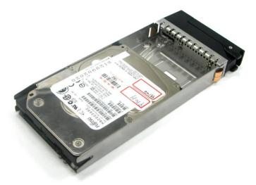
4. Install the mounting screws on the bottom part to secure the drive in the disk tray.
