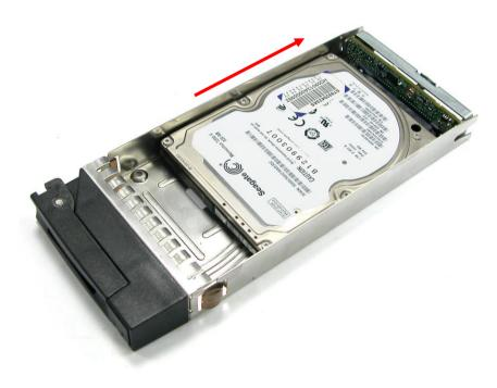
5. Turn the disk tray upside down. To secure the disk drive into the disk tray, tighten four screws on the holes of the disk tray. Note in the picture below where the screws should be placed in the disk tray holes.
