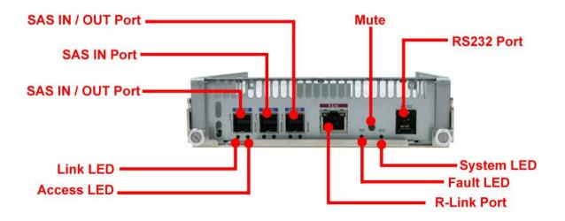
NOTE: SAS IN/OUT Port can be flexibly configured as either SAS IN PORT or SAS OUT PORT by customer's request
