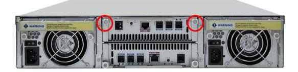
4. Tighten the screws of the Blanking Plate.
