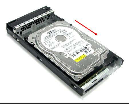
11. Turn the disk tray upside down. Align the four screw holes of the SATA disk drive in the four Hole B of the disk tray. To secure the disk drive into the disk tray, tighten four screws on these holes of the disk tray. Note in the picture below where the screws should be placed in the disk tray holes.
