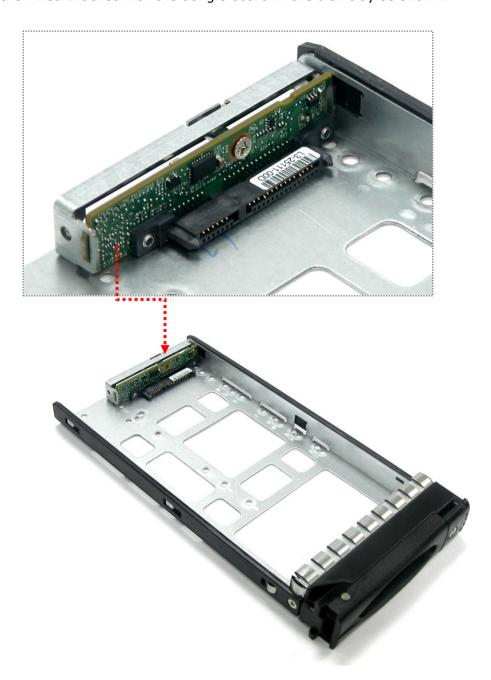
5. Turn the tray upside down. Align the holes of the Fixed Bracket in the two *Hole d* of the disk tray. Tighten two screws to secure the Fixed Bracket into the disk tray.
