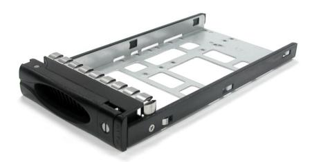
2. Place the disk drive in the disk tray. Turn the disk tray upside down. Align the four screw holes of the disk drive in the four *Hole w* of the disk tray. To secure the disk drive into the disk tray, tighten four screws on these holes of the disk tray. Note in the picture below where the screws should be placed in the disk tray holes.
