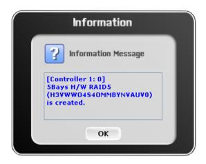
8. The RAID is created successfully. The RAID will be available to the Host/Server immediately and a new disk device will be detected.
