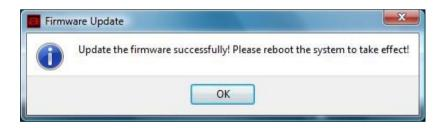
4. Power cycle the RAID subsystem to reboot it. The new firmware will be loaded in the RAID controller. For data security, it is recommended to stop IO to the disk drive (RAID disk) and uninstall/un-mount the RAID disk from the host computer before power cycle.
