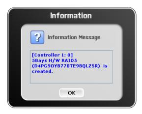
5. The RAID is created successfully. The RAID will be available to the Host/Server immediately and a new disk device will be detected.
