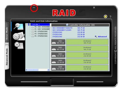
**Close Window** button – Used to close the RAID Manager GUI.
