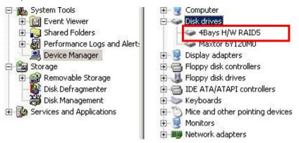
In Microsoft Windows under Device Manager, the new disk drive (4Bays H/W RAID5) is displayed.
