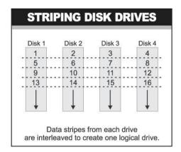
By striping the drives in the array with stripes large enough so that each record falls entirely within one stripe, most records can be evenly distributed across all drives. This keeps all drives in the array busy during heavy load situations. This situation allows all drives to work concurrently on different I/O operations, and thus maximize the number of simultaneous I/O operations that can be performed by the array.
