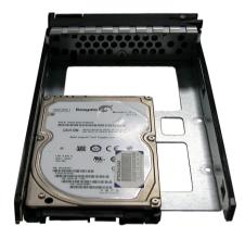
d. Install the mounting screws on the bottom part to secure the drive in the disk tray.
