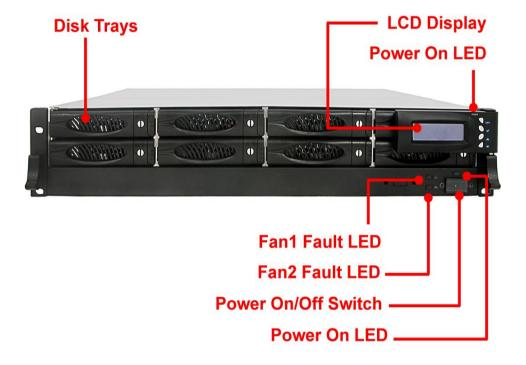
**Power LED** – LED is green when the NAS system in on.
