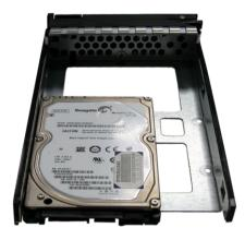
d. Install the mounting screws on the bottom part to secure the drive in the disk tray.
