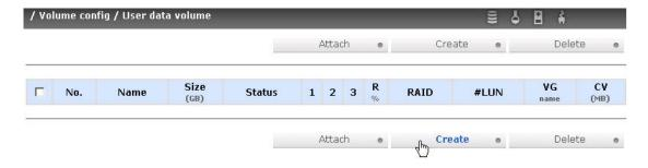
Setup Capacity, Stripe Height, and Block Size for UDV / Volume config / User data volume / Create UDV01 Name: VG name : VG01 ▼ Global ( 136 MB ) 💌 CV No.: Capacity (GB): 2793 I Stripe height (KB): 64 🔻 512 Block size (B): Read/Write: C Write-through cache C Write-back cache Priority: ● High priority
