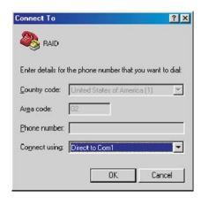
The default setting of the monitor port is 115200 baud rate, 8 data bit, non-parity, 1 stop bit and no flow control.
