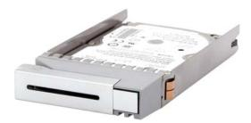
d. Install the mounting screws on the bottom part to secure the drive in the disk tray.
