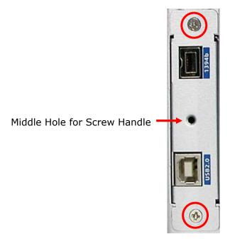
3. Insert the screw handle into the middle hole of the USB/1394 IO interface board and tighten the screw handle.
