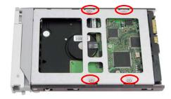
e. Slide the tray into a slot until it reaches a full stop.
