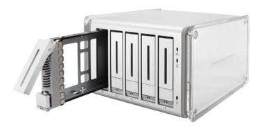
c. Place the hard drive in the disk tray. Make sure the holes of the disk tray align with the holes of the hard drive.
