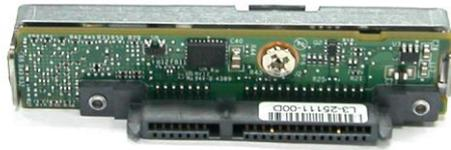
3. Place the dongle board in the disk tray. Turn the tray upside down. Tighten a screw to secure the dongle board into the disk tray.
