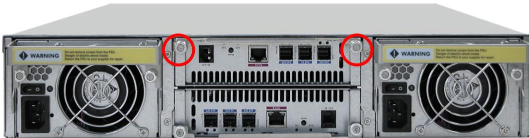
4. Tighten the screws of the Blanking Plate.
