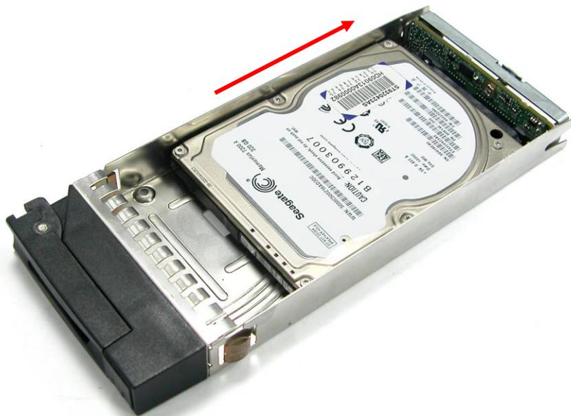
5. Turn the disk tray upside down. To secure the disk drive into the disk tray, tighten four screws on the holes of the disk tray. Note in the picture below where the screws should be placed in the disk tray holes.
