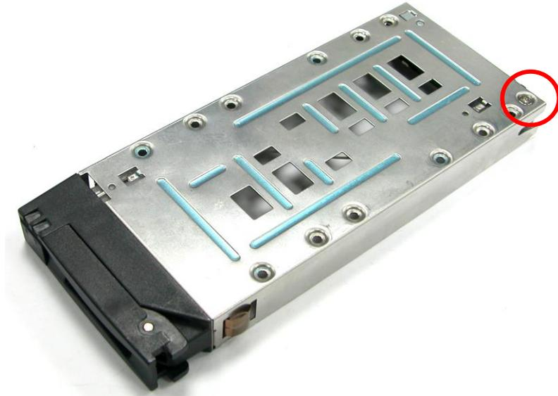
4. Place the SATA disk drive into the disk tray. Slide the disk drive towards the dongle board.
