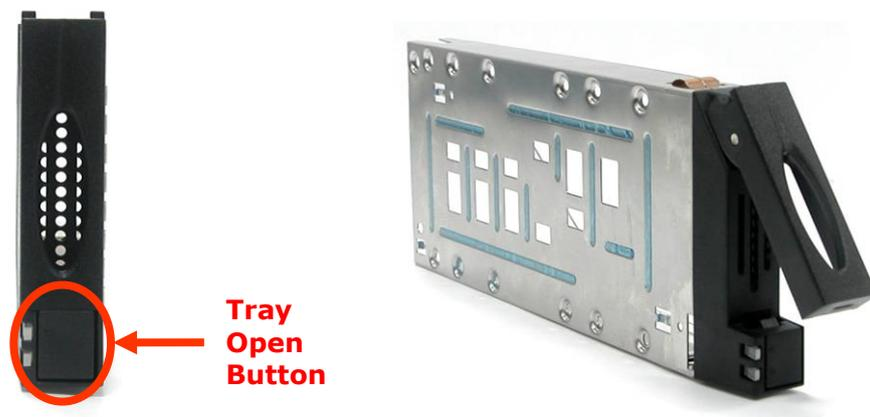
2. Pull out an empty disk tray. Pull the handle outwards to remove the tray from the enclosure.
