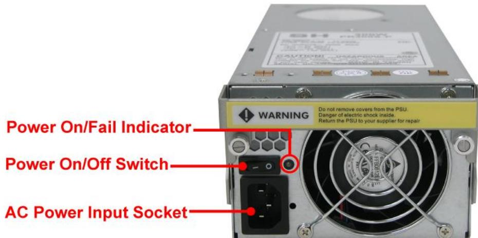
The panel of the Power Supply/Fan Module contains: the Power On/Off Switch, the AC Inlet Plug, and a Power On/Fail Indicator showing the Power Status LED, indicating ready or fail.
