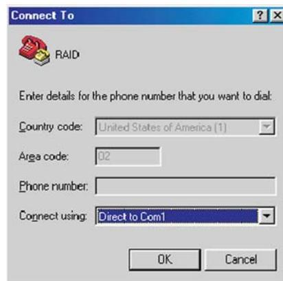
4. The default setting of the monitor port is 115200 baud rate, 8 data bit, non-parity, 1 stop bit and no flow control.
