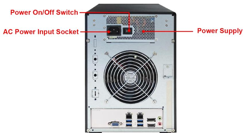
3. To turn on the NAS, press the Power On/Off Switch of power supply at the rear. Then turn on the main switch button in the front panel.
