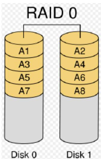
RAID 0 (also called Striping) is the segmentation of logically sequential data, such as a single file, so that segment can be assigned to multiple hard disks in a round-robin fashion and thus written concurrently.
