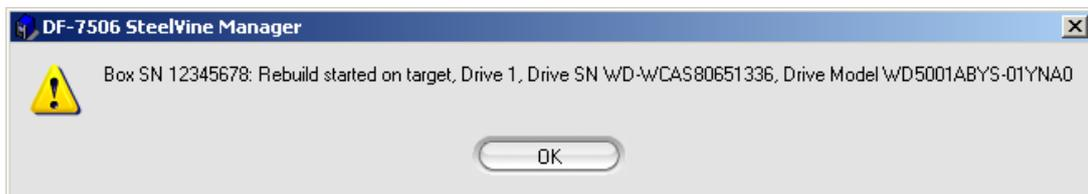
**NOTE: When SAFE (RAID 1) RAID mode is configured, the RAID 1 Volume will undergo Rebuilding and Verification process (initializing the Volume). The RAID 1 Volume is already accessible while initializing.**
