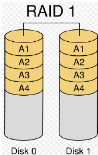
RAID 1 (also called Mirroring) is the replication of data onto the other hard disk in real time to ensure continuous data availability. In a RAID 1 system with two hard disks, the data in one hard disk will be exactly the same as the data in the other hard disk.
