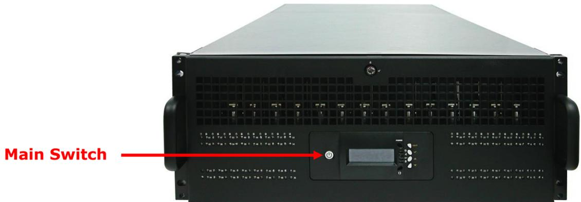
4. Allow the machine a few moments to initialize before using it. The main switch button will continue flashing blue until the system is finished checking each disk slot.
