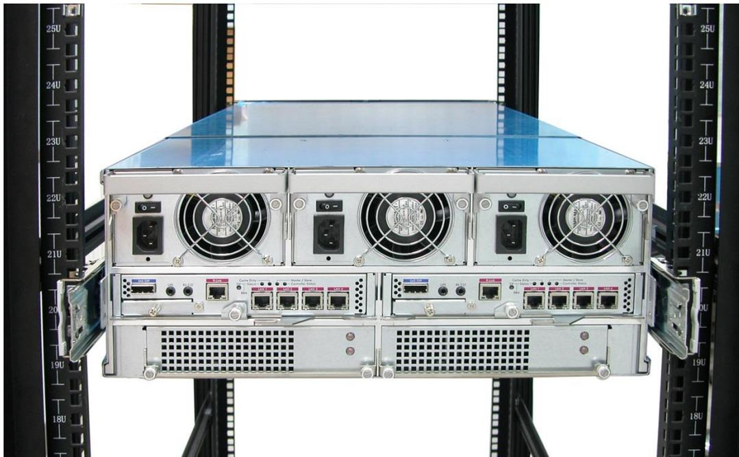
14. Use six (6) M5 screws to lock the enclosure into the rack post, one screw in each corner. Note that the screw driver will need to pass through the corner hole of front panel for the two upper corner holes on both sides.
