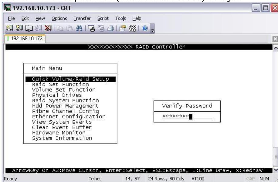
3. After login to Raid System Function menu, select **Update Firmware**. Then choose "Transfer" menu and select "Zmodem Upload List...".
