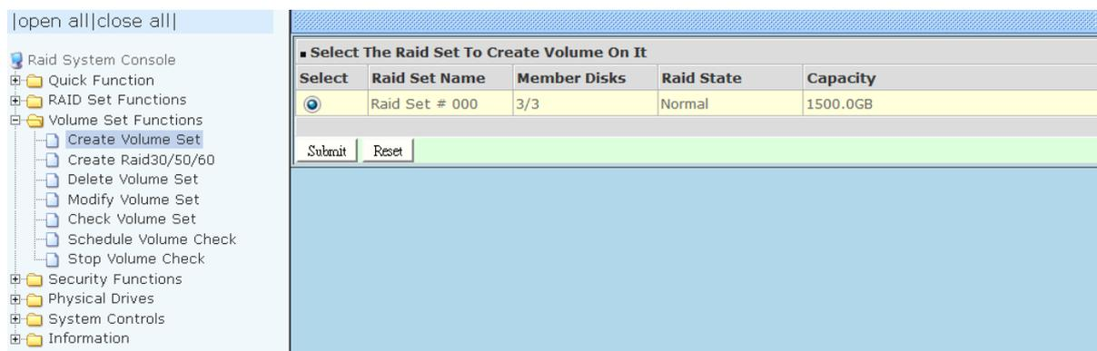
The Volume Set setup screen allows user to configure the Volume Name, Capacity, RAID level, Max Capacity Allowed, Select Volume Capacity, Volume Initialization Mode, Stripe Size, Cache Mode, Tagged Command Queuing, Controller #1 Fibre Port Mapping, Controller #2 Fibre Port Mapping, Fibre Channel/LUN Base/LUN, and Volume To Be Created.
