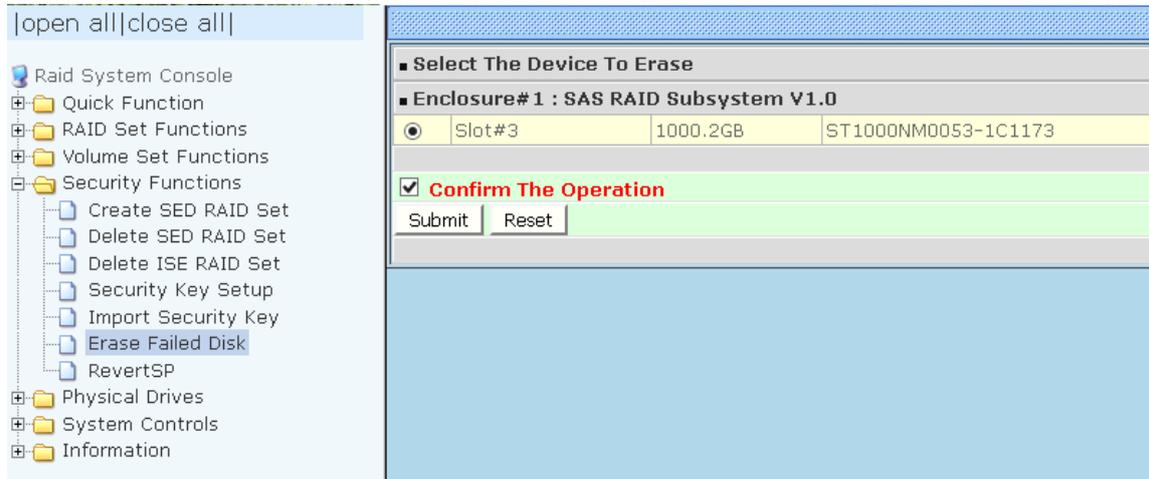
To securely erase the SED or ISE failed disk, choose and click the failed disk Slot# and tick on the "**Confirm The Operation**" and click **Submit**. After secure erase failed disk, there is no way to recover original data.
