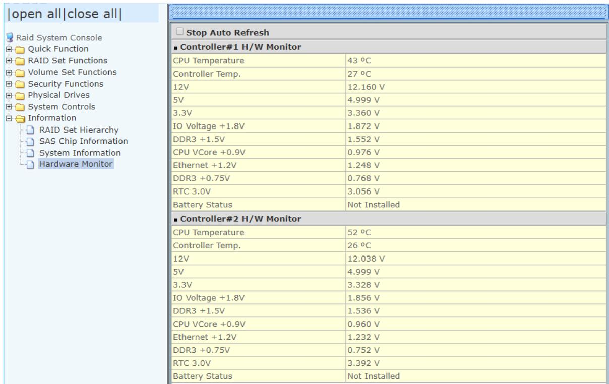
The screenshot shows the Hardware Monitor interface. On the left is a navigation tree with 'Hardware Monitor' selected. The main area displays a table of hardware metrics for two controllers. At the top, there is a checkbox for 'Stop Auto Refresh' which is currently unchecked.
