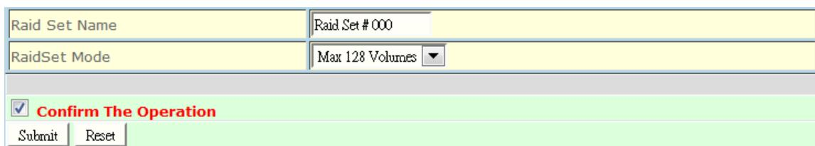
128 volumes is the default mode for SAS RAID controller, the 16 volumes mode is used for support roaming this raidset to SATA RAID controllers. The SATA RAID controller is designed to support up to 16 volumes only. You have to use “Max 16 volumes” on the raidset mode if you plan to roam this raidset between SAS RAID controller and SATA RAID controller.
