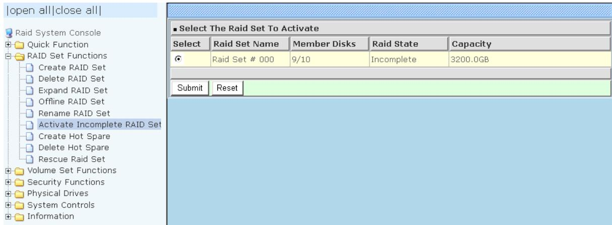
Click on the **Submit** button to activate the Raid Set. The Volume Set(s) associated with the Raid Set will become accessible in “**Degraded**” mode.
