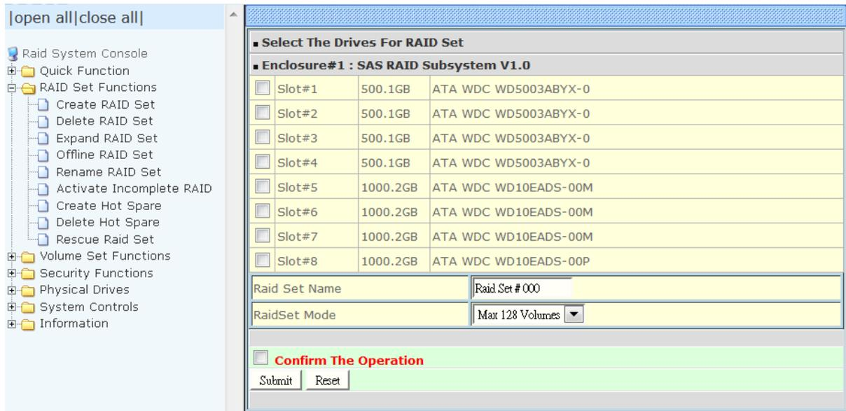
To create a Raid Set, click on the **Create RAID Set** link. A “Select The Drives For RAID Set” screen is displayed showing the disk drives in the system. Tick the box of each disk drive that will be included in Raid Set to be created. Enter the preferred Raid Set Name (1 to 16 alphanumeric characters) to define a unique identifier for the Raid Set. Default Raid Set name always appear as **Raid Set # xxx**.
