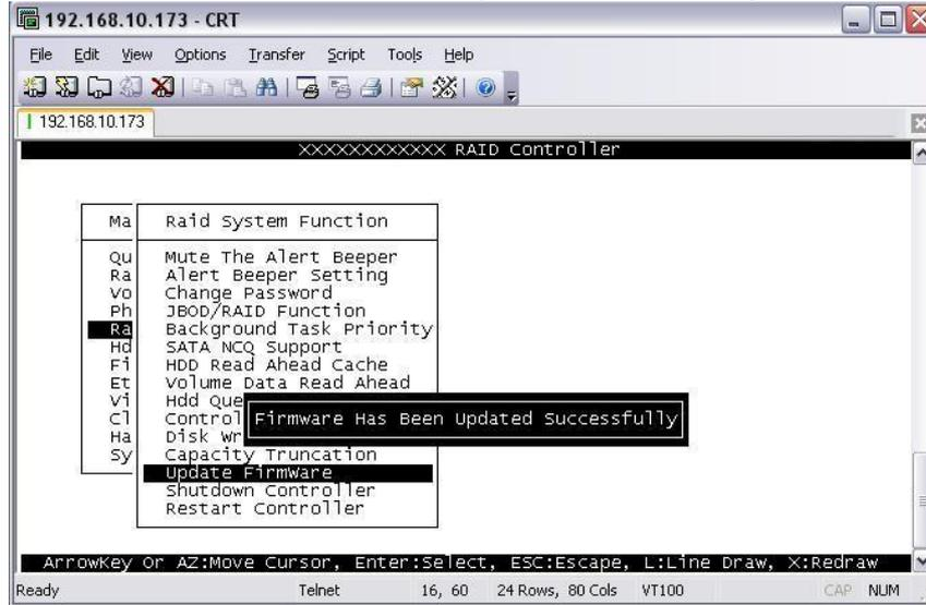
10. The RAID Controller must be restarted in order for the new firmware to take effect.
