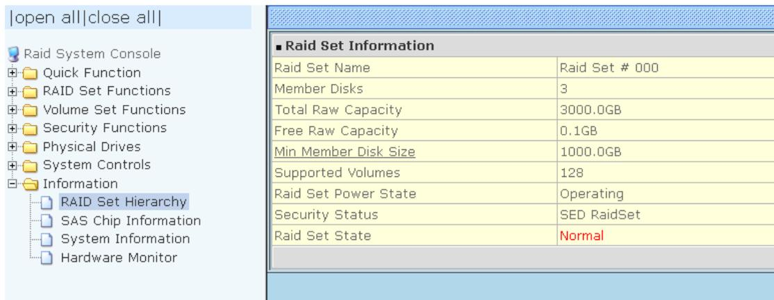
The Raid Set Hierarchy can show SED Raid Sets, click the Raid Set name link and check the Raid Set Information for Security Status:
