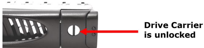
When the Lock Groove is vertical, then the Drive Carrier is unlocked.
