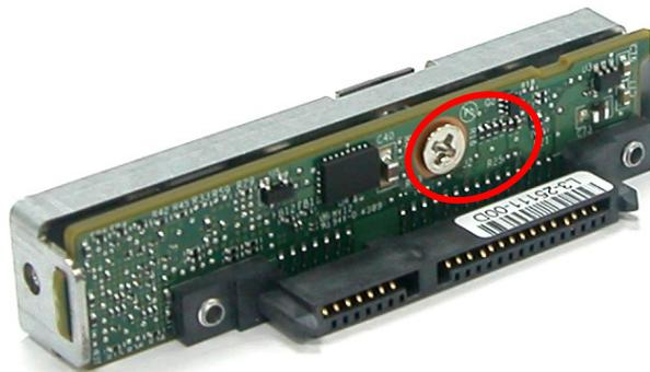
8. Place the Fixed Bracket with the dongle board in the disk tray as shown.
