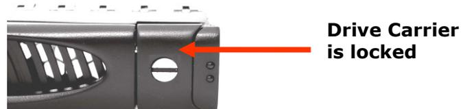
When the Lock Groove is horizontal, this indicates that the Drive Carrier is locked.
