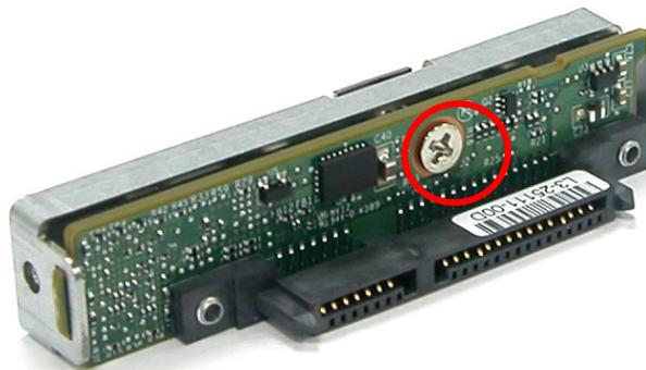
4. Place the Fixed Bracket with the dongle board in the disk tray as shown.
