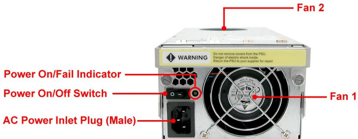
The panel of the Power Supply/Fan Module contains: the Power On/Off Switch, the AC Inlet Plug, and a Power On/Fail Indicator showing the Power Status LED, indicating ready or fail.
