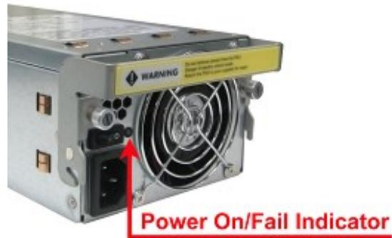
When the power cord connected from main power source is inserted to the AC Power Inlet, the power status LED becomes **RED**. When the switch of the PSFM is turned on, the LED will turn **GREEN**. When the Power On/Fail LED is **GREEN**, the PSFM is functioning normally.
