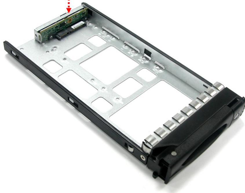
5. Turn the tray upside down. Align the holes of the Fixed Bracket in the two *Hole d* of the disk tray. Tighten two screws to secure the Fixed Bracket into the disk tray.
