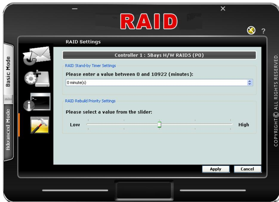
**RAID Stand-by Timer Settings** – Use this option to select time option, in minutes, before the RAID comes into stand-by mode. When there is no host access to the RAID, after the preset time (minutes), the RAID will be in standby mode.
