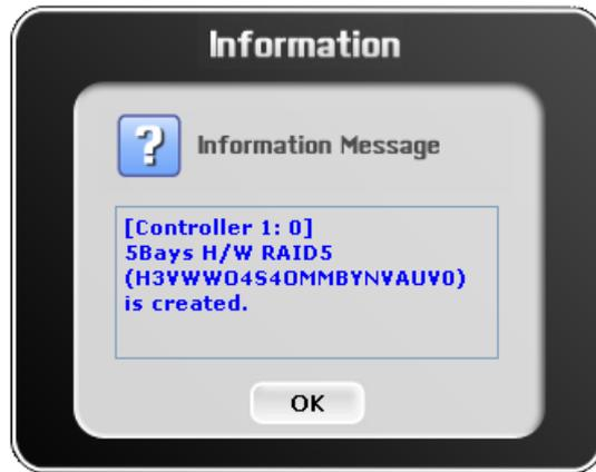
8. The RAID is created successfully. The RAID will be available to the Host/Server immediately and a new disk device will be detected.
