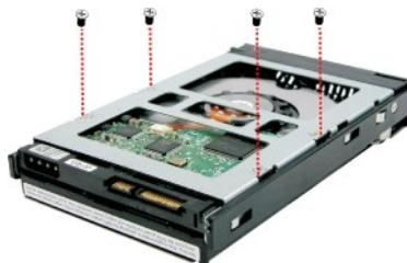
5. Insert the disk tray with disk drive in the disk slot.
