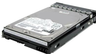
4. Tighten the mounting screws to secure the disk drive into the disk tray.
