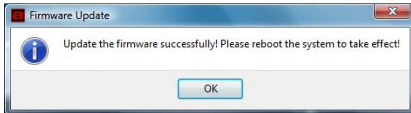
4. To reboot the RAID subsystem, uninstall the disk drive from the host system then power cycle the RAID subsystem. The new firmware will be loaded in the RAID controller.
