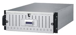
The EP-4423 series RAID subsystem features 8Gb or 4Gb FC-AL host performance to increase system efficiency and performance. It features high capacity expansion, with 42 hot-swappable SAS/SATA II hard disk drive bays in a 19-inch 4U rackmount unit, scaling to a maximum storage capacity in the terabyte range. The EP-4423D series also supports dual controllers which provide better fault tolerance and higher reliability of system operation.
