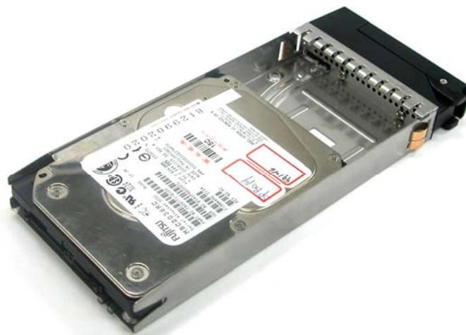
4. Install the mounting screws on the bottom part to secure the drive in the disk tray.
