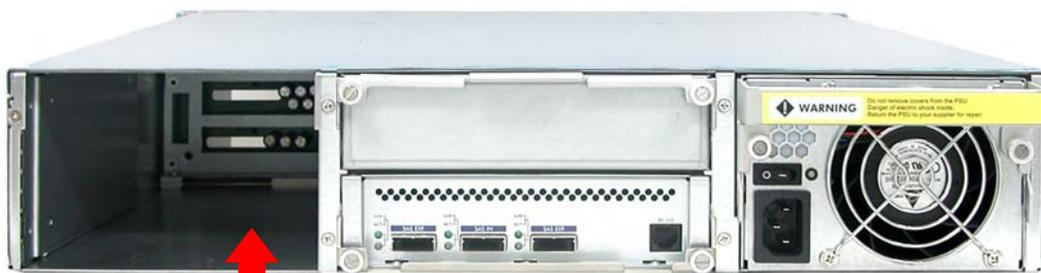
**Power Supply Fan Module Plate Cover**
