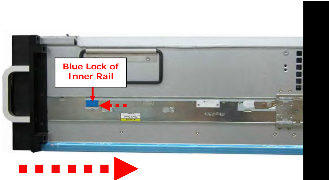
View from Right Side of Enclosure Blue Lock of Inner Rail is Pushed a Little Outwards and Enclosure is Pushed Inwards
