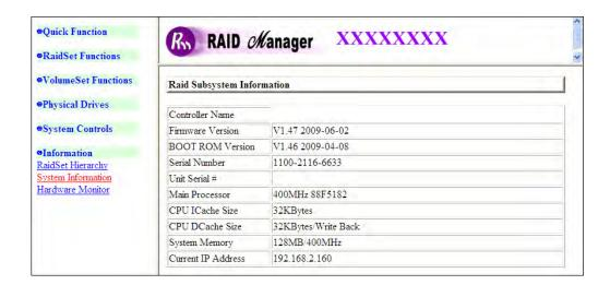
The controller name, firmware version, serial number, main processor, CPU data/instruction cache size and system memory size/speed appear in this screen.
