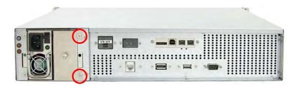
2. Remove the cover plate and insert power supply carefully. Tighten two screws to lock the power supply in place.
