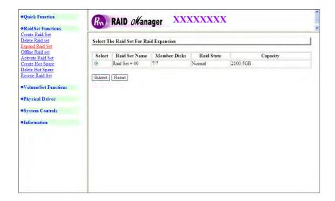
To expand a Raid Set, click on the **Expand Raid Set** link. Select the Raid Set which you want to expand.
