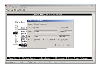
7. When the firmware downloading is completed, the confirmation screen appears. Select Yes to start programming the flash ROM.
