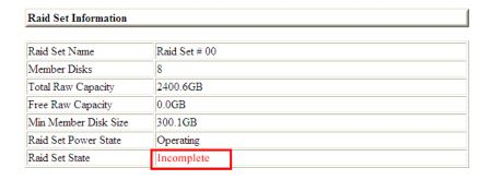
The Volume Set will not be visible and the failed or removed disk will be shown as "Missing".
