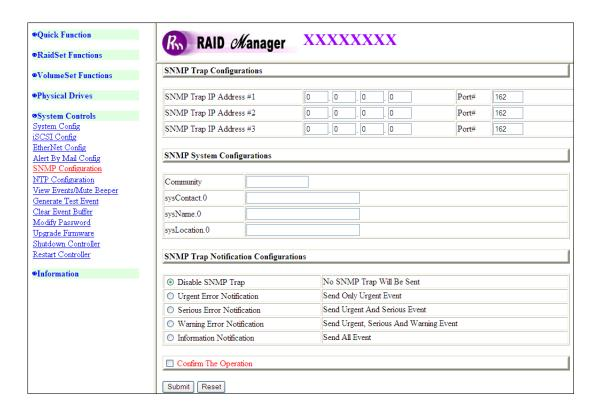
**SNMP Trap Configurations:** Type the SNMP Trap IP Address. The SNMP Port is set to 162 by default.
