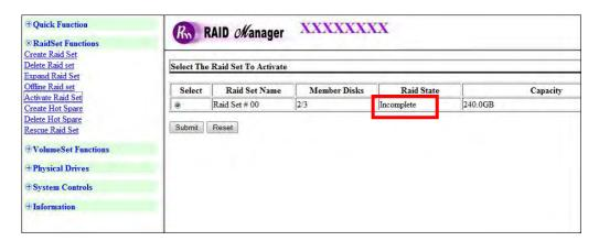
Click on the **Submit** button to activate the Raid Set. The Volume Set(s) associated with the Raid Set will become accessible in "**Degraded**" mode.
