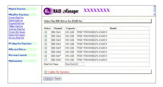
To create a Raid Set, click on the **Create Raid Set** link. A "Select The IDE Drives For RAID Set" screen is displayed showing the IDE drives in the RAID subsystem. Check the "Select" option to include a physical drive to the current Raid Set. Enter the preferred Raid Set Name (1 to 16 alphanumeric characters) to define a unique identifier for the Raid Set. The default Raid Set name will always appear as Raid Set # 00 for first Raid Set.
